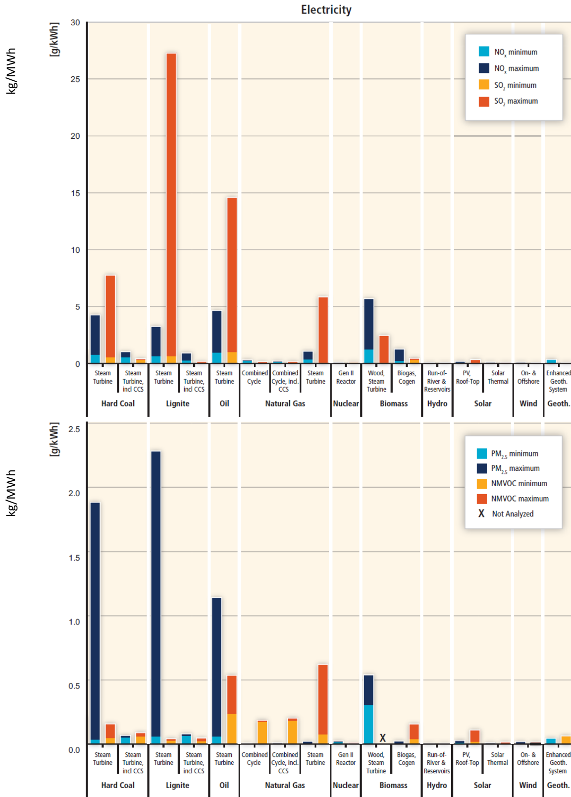
Figure E.2. Life Cycle Emissions of Air Pollutants from Electricity Generation. 551
